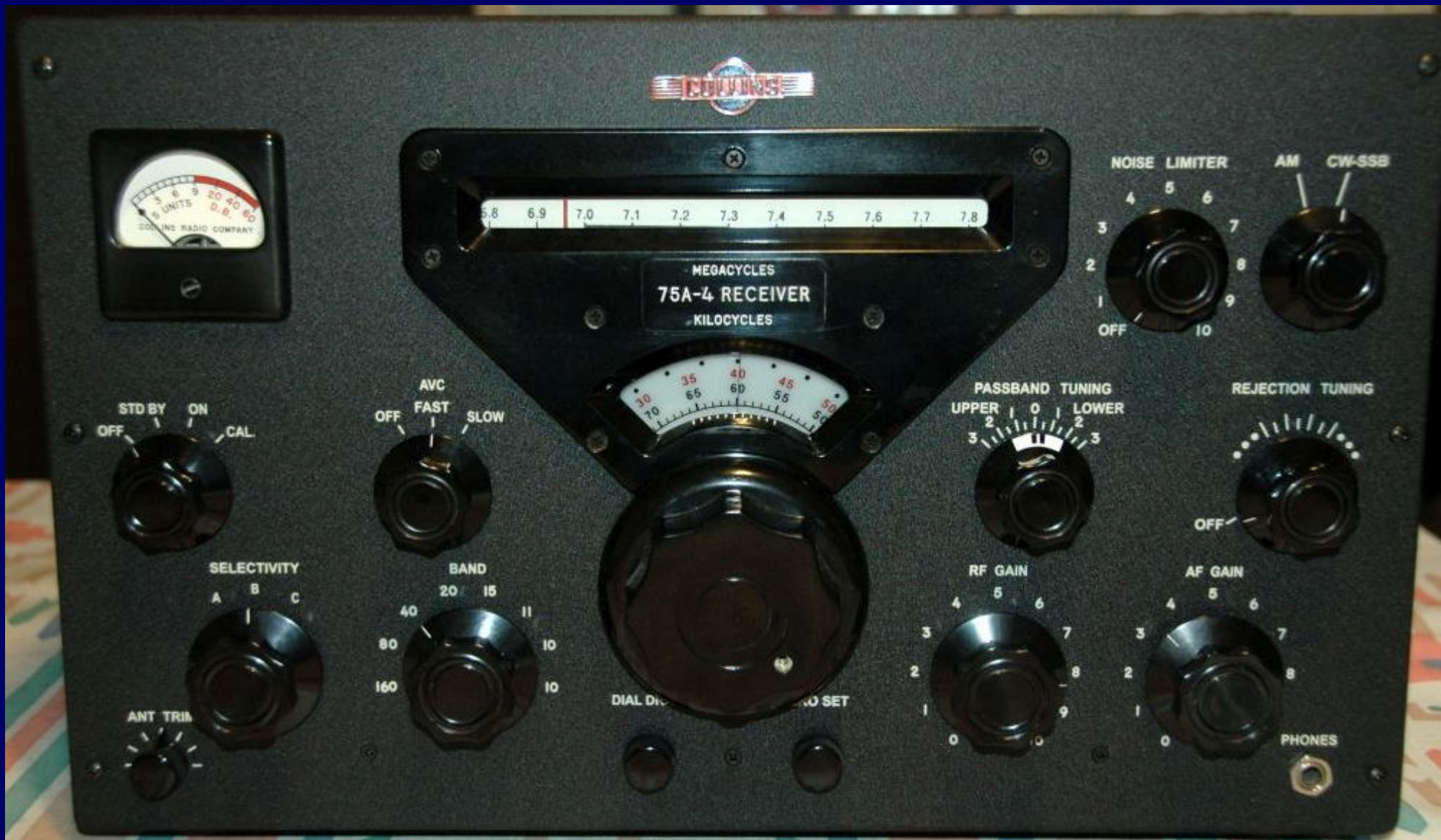
Dual Conversion Superhet Receiver "Boat Anchor" from 1955 Collins Receivers, Transmitters, and Transceivers still attract top dollar at Flea Markets and on line Swap Shops.
