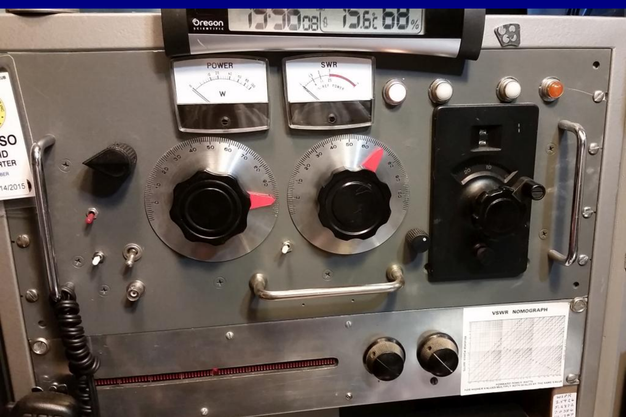
VE3GSO SWR/Power Meter, C-L-C Antenna Tuner, Antenna Switch
